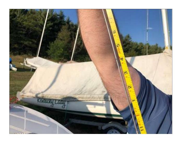
Step 5: Forestay tension is about 80-110 lbs, based on 1/8inch wire we try to hit 9-12 on the gauge.
