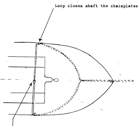
NOTE: Snap & ring connection on centerline of boat.
