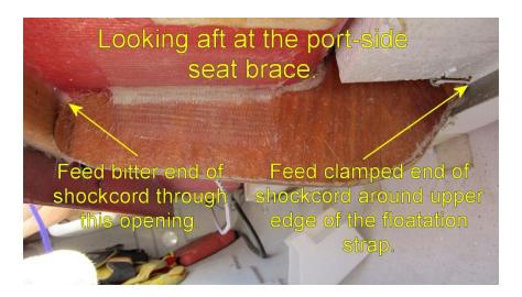
Feed the bitter end of the shockcord through the clamped end and tie a stopper knot:
