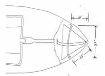
2. Lay the uninflated air bag in the bow to be sure the position of the blocks is correct.
